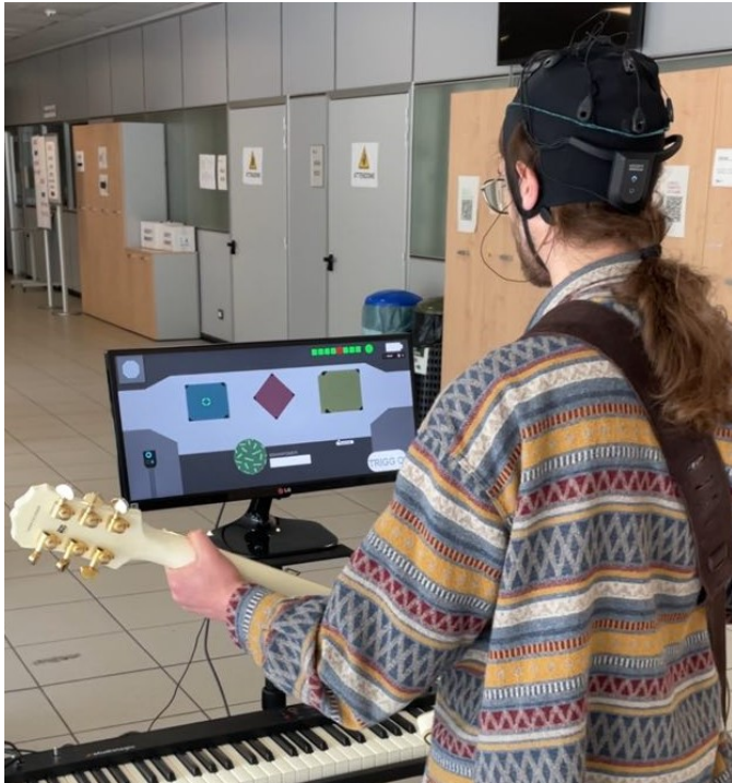
Fig. 1: The guitarist testing the BCI commands using Unicorn Hybrid Black EEG headset.
